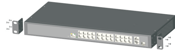
Figure 2-1 Install hangers diagram
