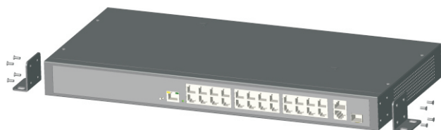
Figure 2-3 Hangers installation diagram
