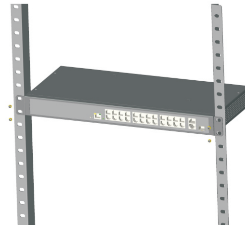
Figure 2-2 Install switch to the rack
